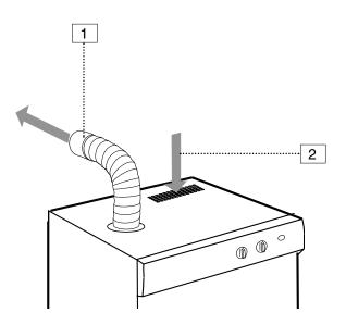
The drying cabinet permanently installed and connected to the evacuation duct
